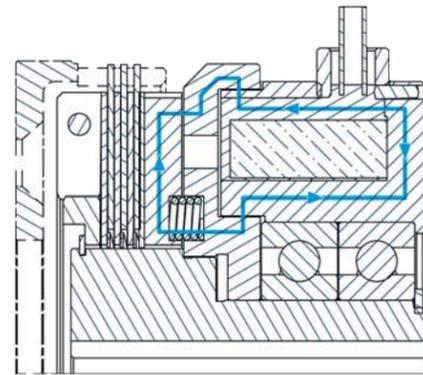
Radial magnetic flux path provides maximum torque throughout life of clutch.
